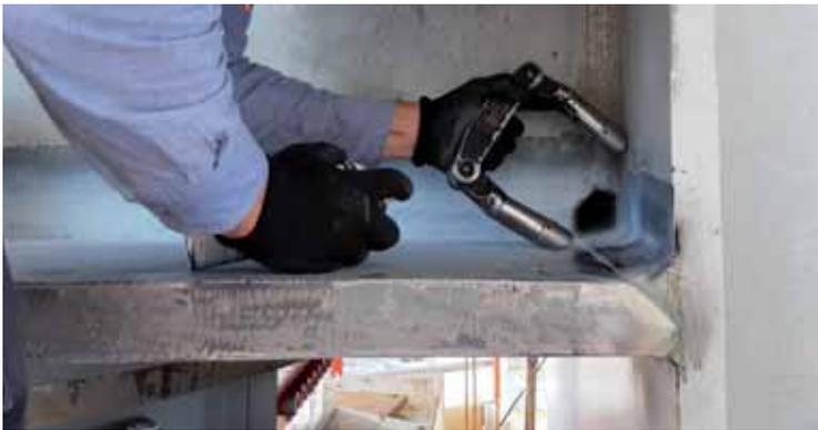
Fig. 41 - Controllo magnetoscopico
